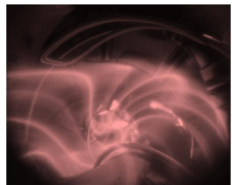
Figure 3: View from re-entrant viewport showing light emitted from electron beams confined on magnetic field lines in H-1NF.
