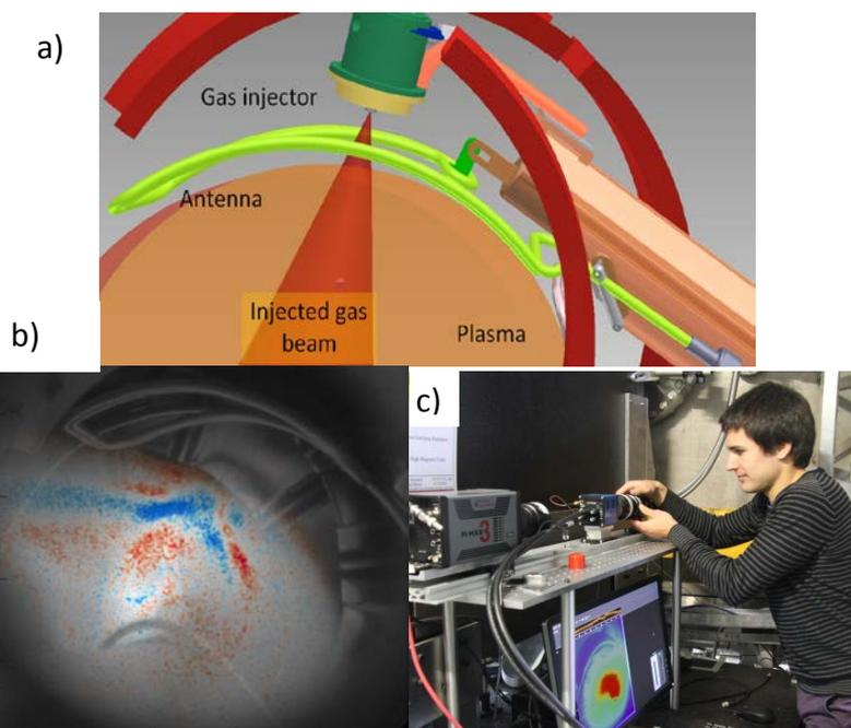
Figure 1: a) arrangement of the gas puff injector (green), RF antenna (lime green) and plasma b) Snapshot of wave structure travelling away from the loop antenna above. Wave crests are red, troughs are blue. c) PhD student Alex Thorman aligns the high speed camera viewing the antenna.
