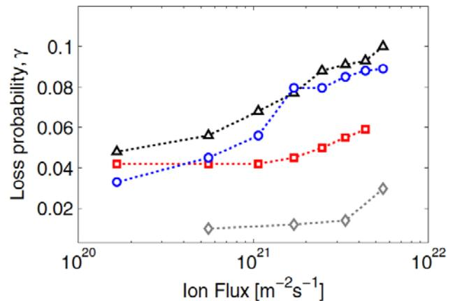
Figure 2: Loss probabilities measured in the early afterglow for tungsten (black triangles), graphite (blue circles), stainless steel (red squares) and for control case (grey diamonds)
