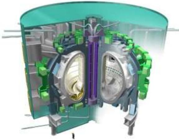
Inside the ITER cryostat showing magnets and vacuum vessel with protective tiles and divertor added to the left side (published with permission of ITER)
