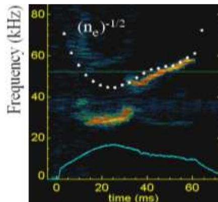
Figure 2 Frequency-time diagram of magnetic fluctuations in H-1NF showing the plasma density  $n_e$  in blue, and Alfvénic scaling with  $1/\sqrt{n_e}$  (white).
