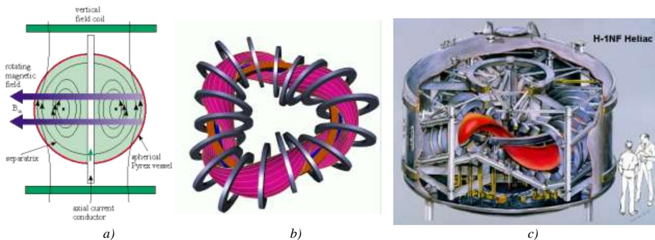
Figure 1 a) The Rotamak spherical torus showing indicative magnetic field lines
