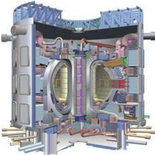
Cutaway view of cryostat showing magnets and vacuum vessel (published with permission of ITER)
